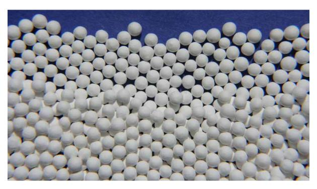
KELTEC Technolab Activated Alumina Desiccant is highly porous with a large surface area, which will not weaken or break when subjected to high liquid concentrations. High crush strength and strong, durable shipping bags, allow for easy transport.
