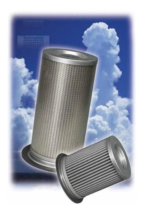
One common method of increasing the capacity of a given sized air-oil separator is through the use of pleated filter media. In this case, the filter media is processed through a machine whereby the normally flat surface is "pleated" or induced into a wave-like appearance. A separator configured in this manner can then be suited for approximately 2x the air flow capacity, as that of a standard air-oil separator, manufactured in the standard, wrapped method.
