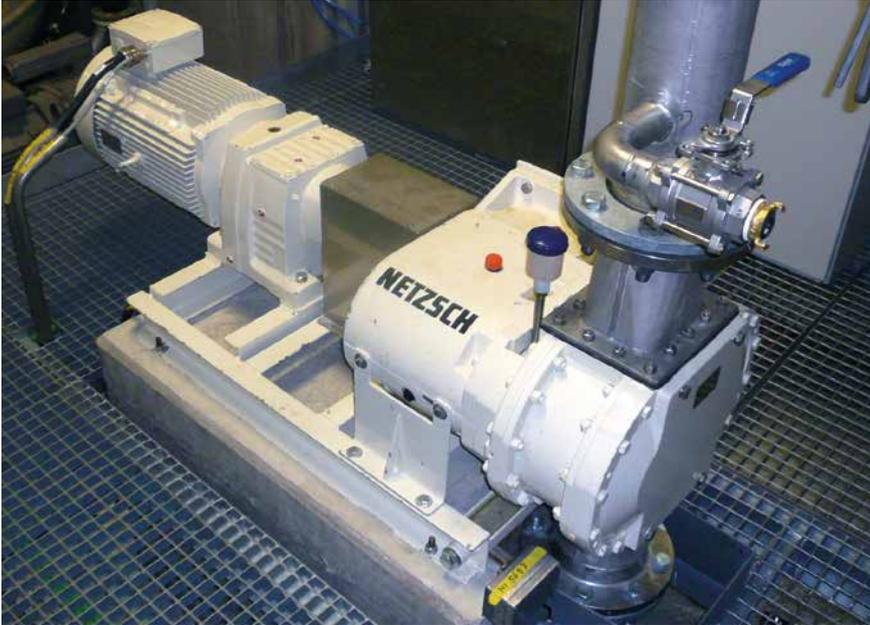
A TORNADO® pump in a paper factory for unloading Kaolin from tankers. Flow rate is 75 m<sup>3</sup>/h and pressure is 4 bar.
