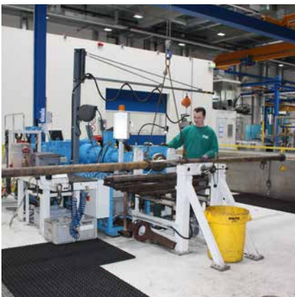
Extruder with stator for oil production
