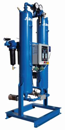
The Aircel BHD Series is a fully automatic breathing air system that utilizes a unique dual tower regeneration process. The BHD Series purifies compressed air to breathable air by removing a variety of contaminants including dust, dirt, water, oil, hydrocarbon vapor, and dangerous levels of carbon monoxide.
